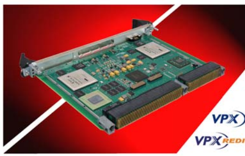
Curtiss-Wright's first FPGA-based 6U VPX/VPX-REDI engine, the CHAMP-FX2, features Dual Xilinx Virtex-5 FPGAs.
